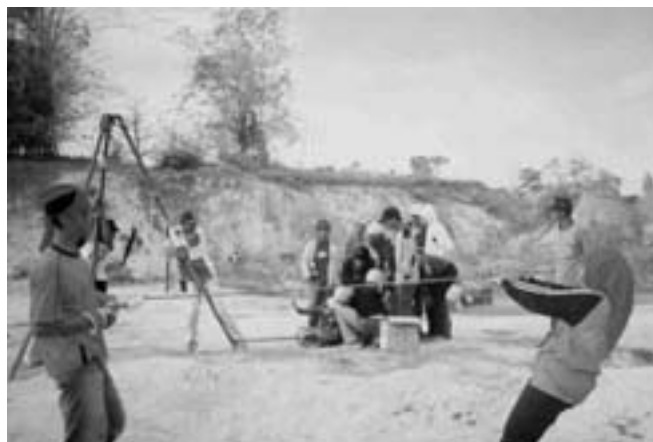
Fig. 6: Institute of Technology at Surabaya (ITS) acquiring refraction seismic data with student power to hoist the "thumper" source.
