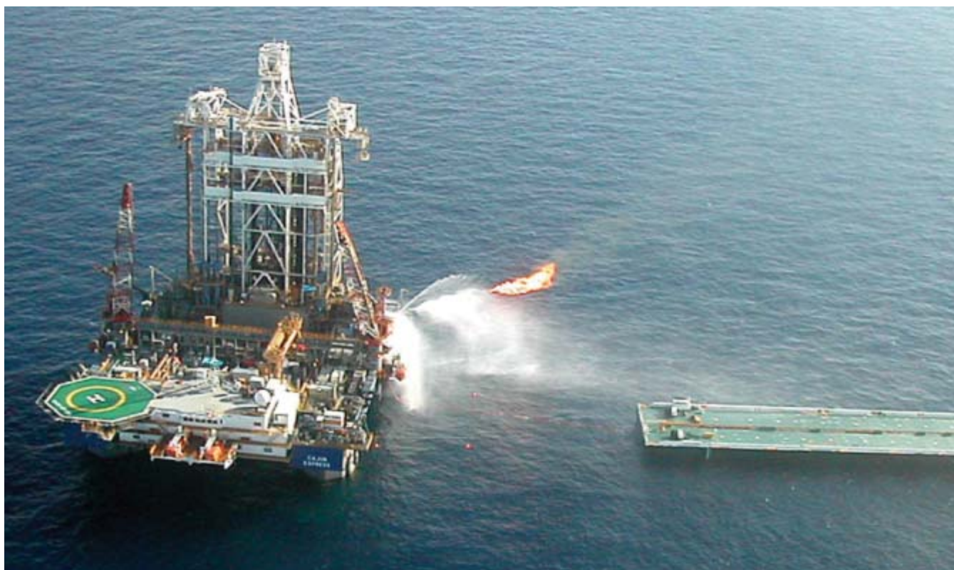
Figure 2. The rig Cajun Express conducts the Tahiti GC 640 well test in August 2004.
