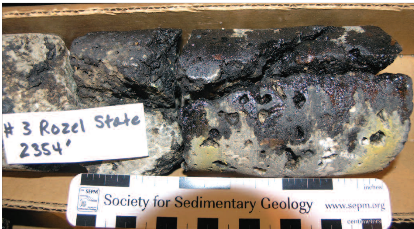
Figure 1: Whole core from the Amoco #3 West Rozel, Utah, taken at 2,354 ft. Note heavy oil staining along fractures.
