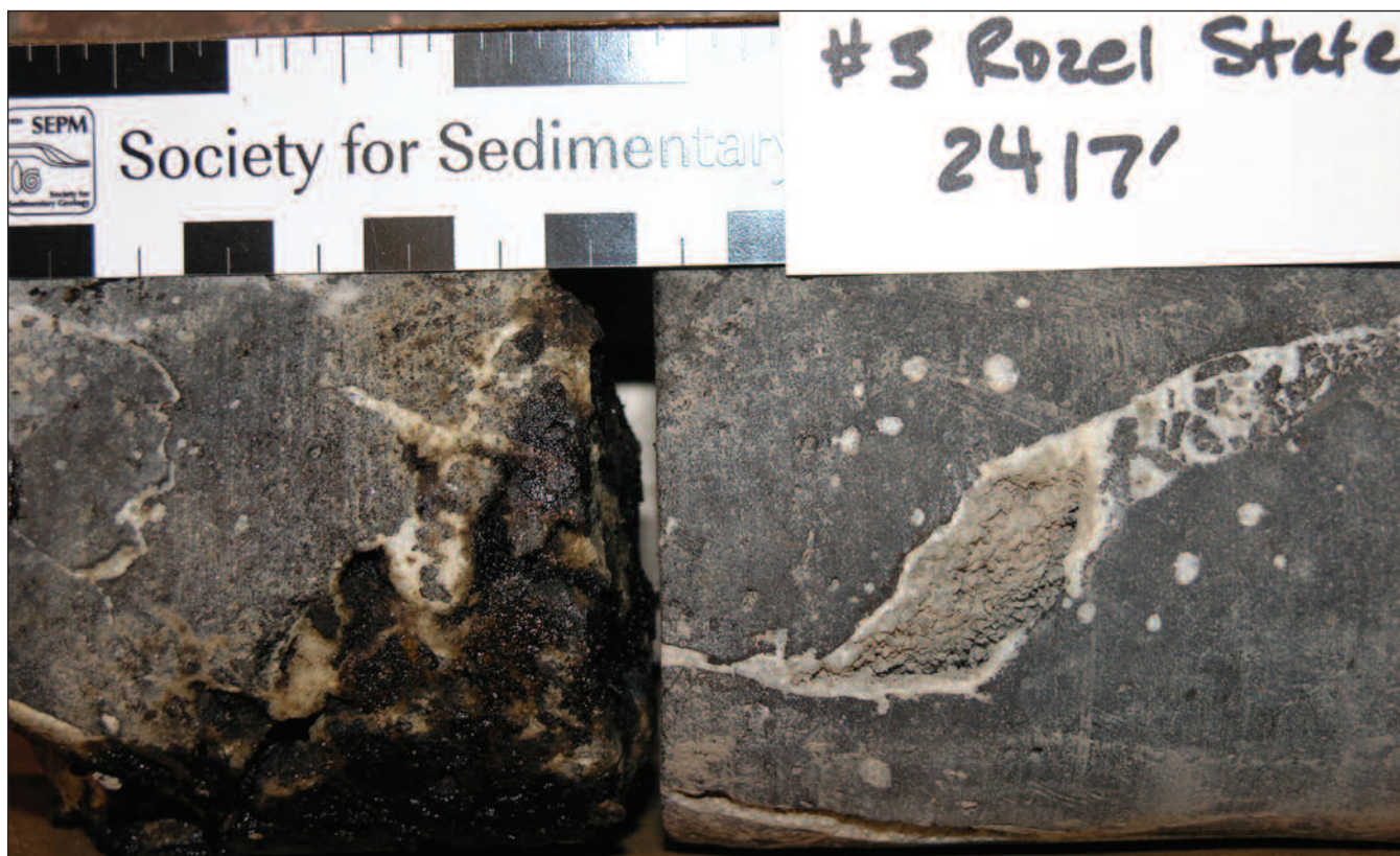
Figure 2: Whole core from the Amoco #3 West Rozel, Utah, taken at 2,417 ft. Note white mineralization filling vesicles and old fractures appears to have precluded oil staining seen above.
