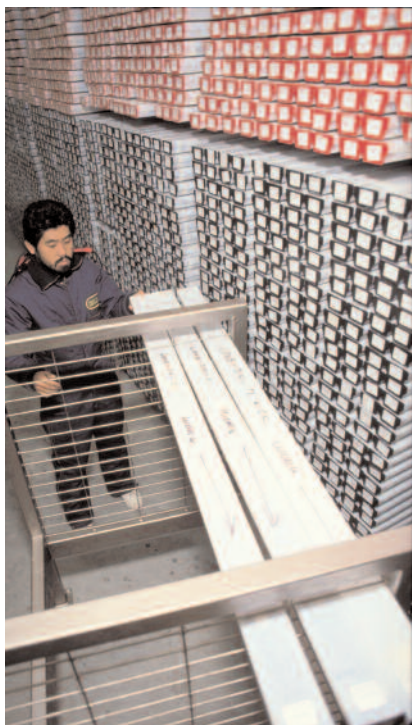
Figure 6 Inside the Gulf Coast Repository core warehouse at Texas A&M. The deep sea sediment cores are stored at 40°F to preserve them.
