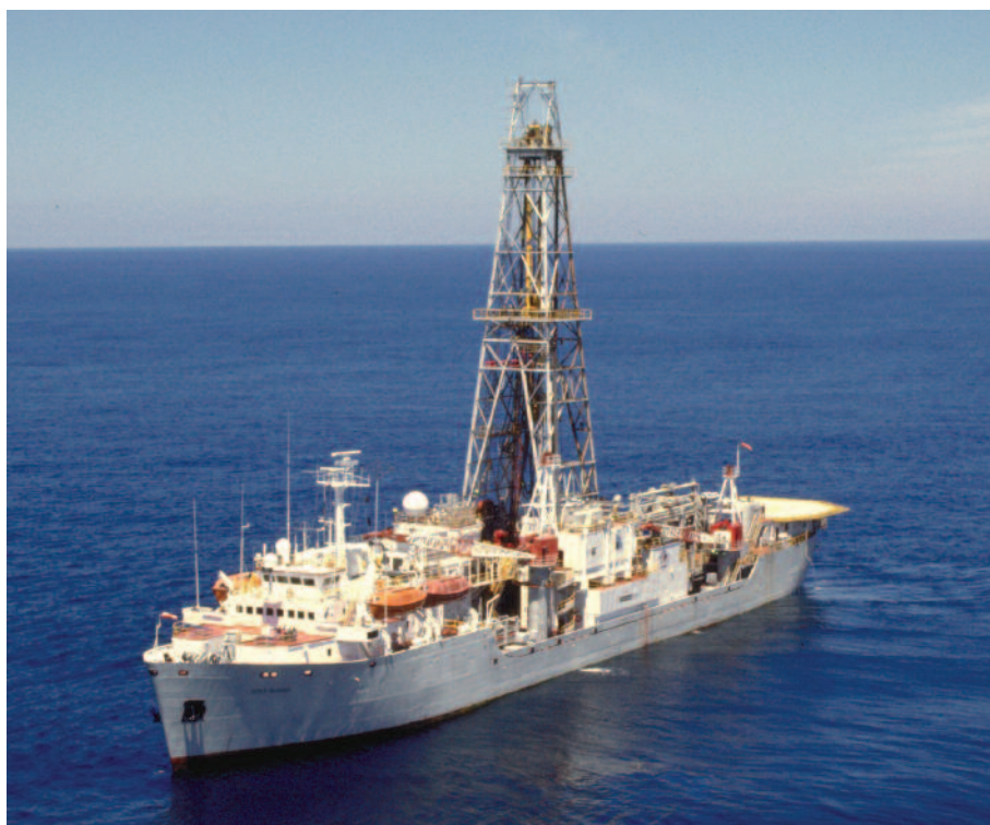
Figure 4 The drillship JOIDES Resolution at sea. The Resolution replaced the Glomar Challenger in the 1980s and will be replaced by the high-tech drillship Chikyu in the future. The Resolution can take deep sea cores in 20,000 ft of water using riser-less drilling.
