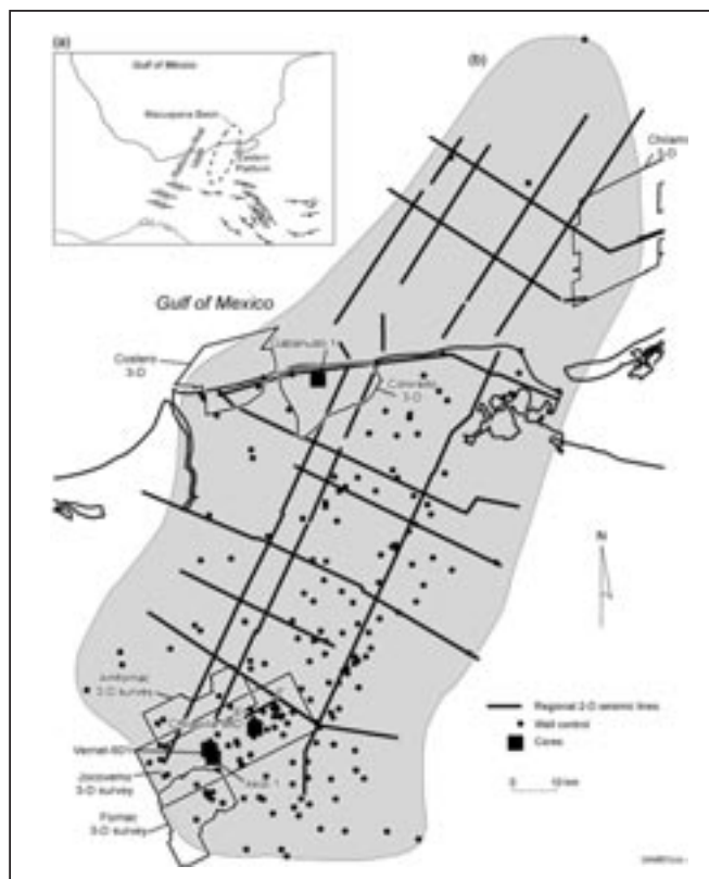
Fig. 1. (a) Location of the Macuspana Basin, with structural elements. (b) Well control and distribution of 3-D surveys and principal 2-D seismic lines used in the study.
