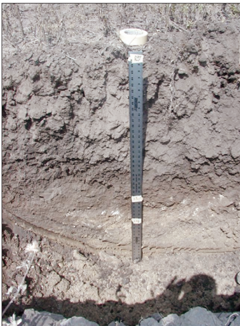
Figure 1: Top of naturally occurring soil profile in the study area. Quantitative characterization of these soils, particularly mineral and chemical composition variation with depth, provided essential data for determining the oil and gas development activities that could cause adverse impact.
