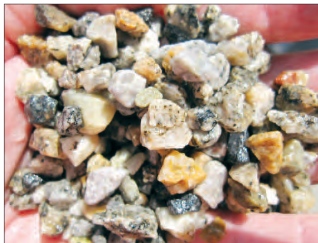
Drill cuttings from a depth of 900 feet in the Pleistocene alluvium of the San Fernando Valley, California.
