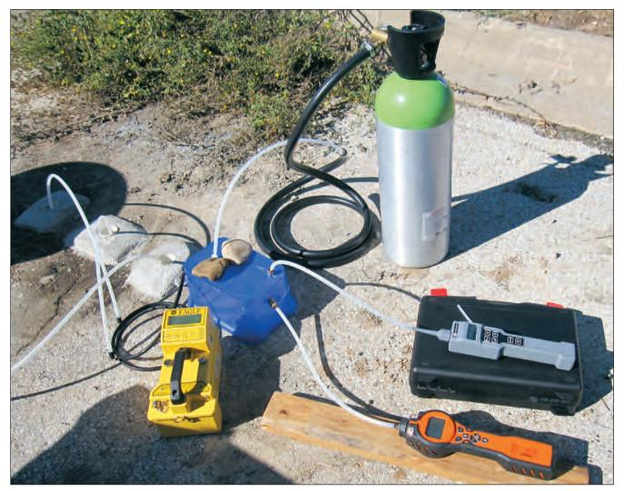
Leak detection testing using helium gas
