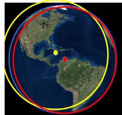
Figure 5: Depicts approximate geocentric datum locations and shift example (yellow circle: NAD 1983 and red circle: WGS 1984. Origin of each is offset, thereby producing different geographic coordinate locations.
