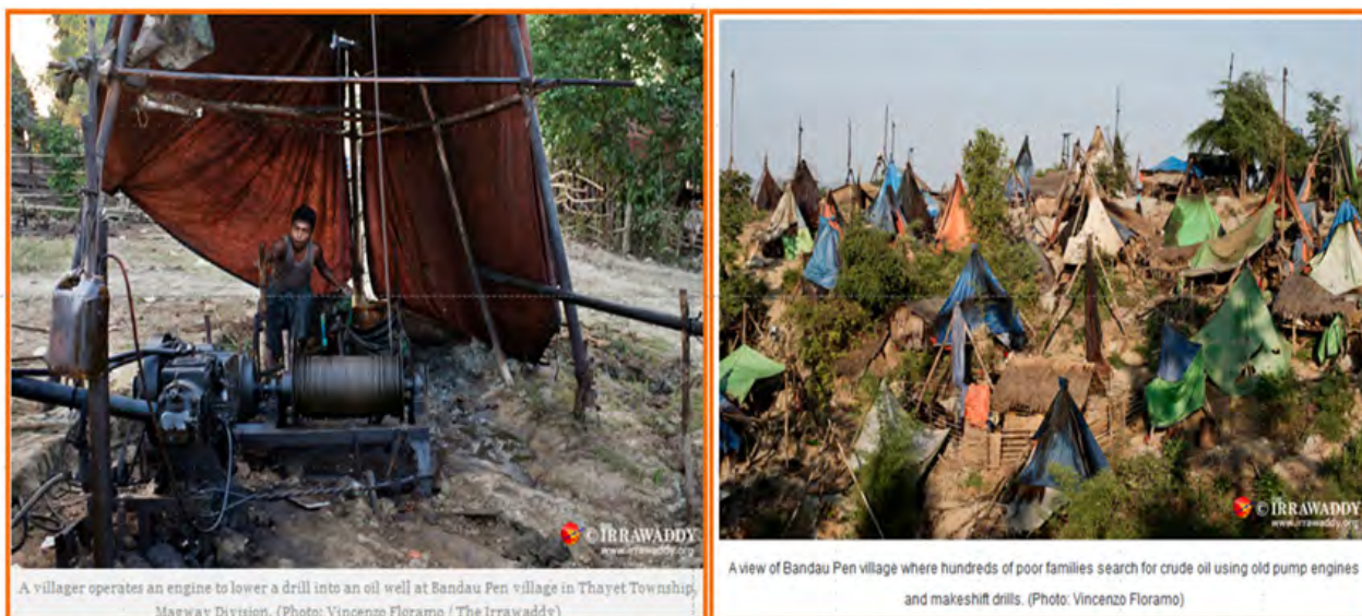
Figure 9. Local oilfield operations onshore Myanmar include the use of handmade rotary drilling rigs (Irrawaddy Times, 2013).
