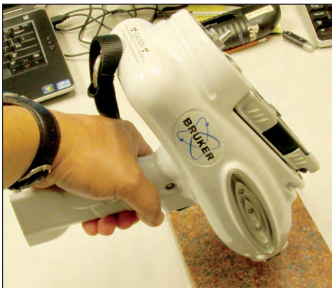
Bruker Tracer IV portable X-ray fluorescence (pXRF) spectrometer
