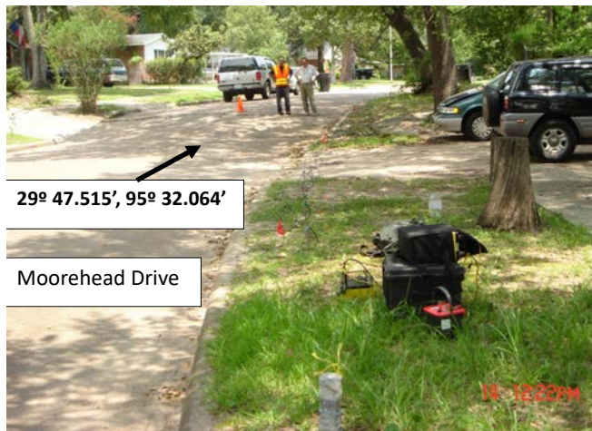
Figure 4. Picture showing coordinates of the Long Point fault, the fault scarp on the road and the location of resistivity profile. The view is to the north.
