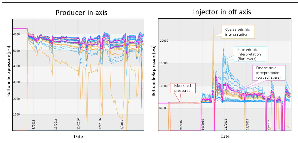
Figure 7. Comparison of actual bottom hole pressures (red circles) and simulated pressures for various scenarios (colored lines) over six months. These results indicated that the coarse-scale seismic interpretation (yellow lines) produced pressures that were too low, suggesting the models were too disconnected. Using curved layers in the fine scale seismic interpretation (pink lines) produced a better match between modeled and actual pressures.
