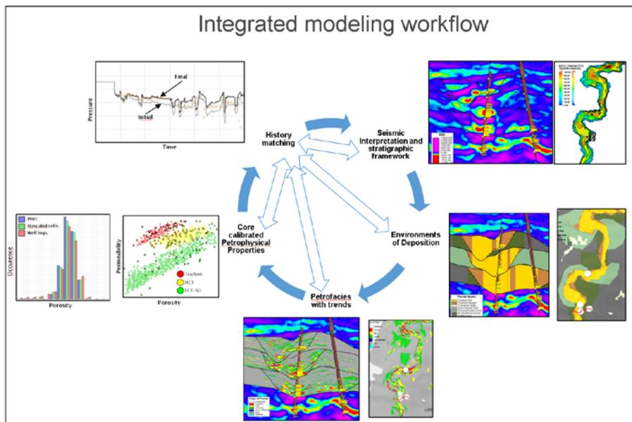
Figure 5. Integrated modeling workflow illustrating the loop from seismic interpretation to static modeling to dynamic simulation and the feedback provided by history matching to update the seismic interpretation and static model.
