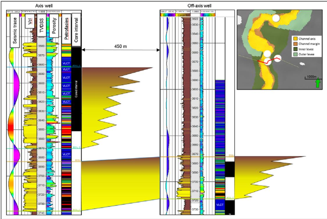
Figure 3. Wells inside and outside the channel axis show a highly variable net to gross.
