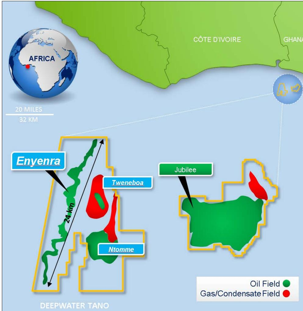
Figure 1. Location map for Enyenra field. The field is located 60 km off the coast of Ghana and 25 km west of the Jubilee field. From the northernmost to southernmost wells, the field extends 24 km and varies in width from 300-1000m.
