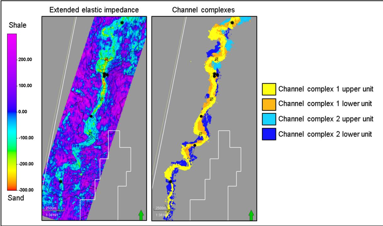
Figure 2: Sum of negative amplitudes extracted from an extended elastic impedance volume showing possible sand distribution. Four channel complexes were identified on seismic data and verified with static pressure data.
