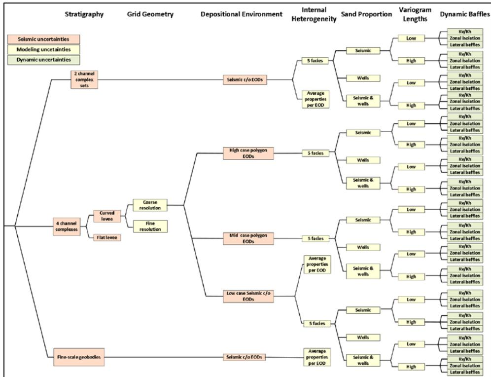
Figure 4. Decision tree illustrating the seismic, modeling, and dynamic uncertainties considered in model construction.
