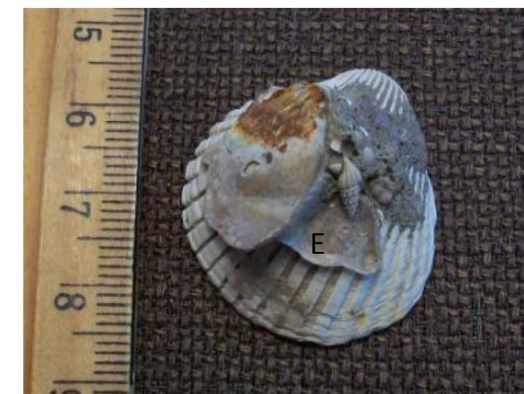
E= Encrustation C= Corrosion
