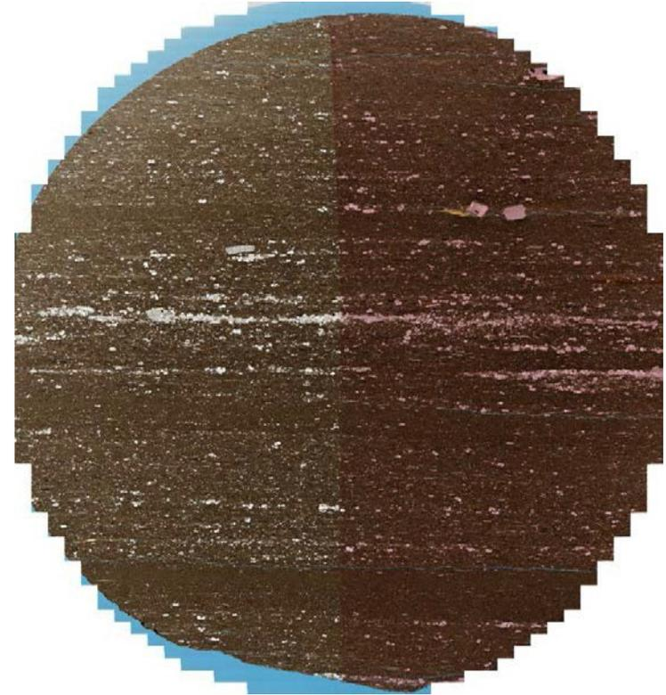
The transmitted light image of the twin thin section surface allows inferences regarding depositional setting to be made.
