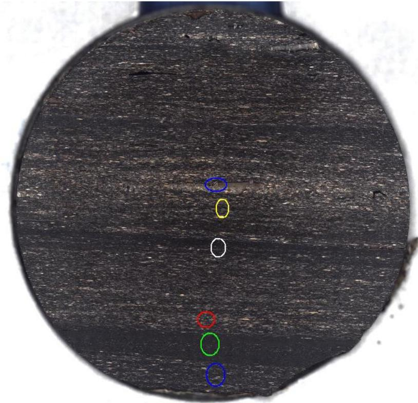
The reflected light image of the ion milled surface illustrates porosity, mineralogy, and TOC differences and enables ROI selection
